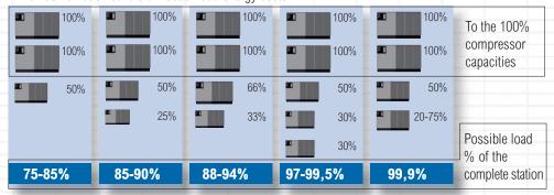
... irrespective of the combination of compressors, **Airleader** gets the best out of every combination as well as reducing operating pressure to a minimum. An improved graduation insures less motor starts and load changes of the compressors.
