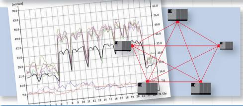
There is no longer a fixed priority or sequence. Your production determines the correct combination of compressors, to ensure the most efficient combination of compressors runs for the actual air consumption. Same size Compressors are allocated the same operating hours.
