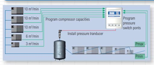
... and **Airleader** will combine compressors of different sizes to form a unit that automatically adjusts itself - in line with the current compressed air consumption - to the production requirements. It ensures that always the most efficient compressor combination generates the compressed air required.
