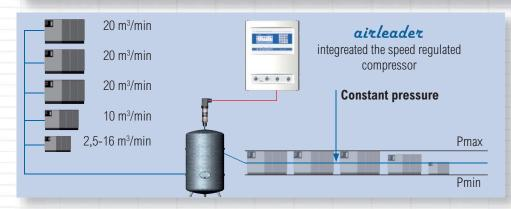
The control strategy automatically ensures that, compressors connect or disconnect step less within the pressure band. An exceptionally low switching frequency protects the compressors and prolongs their service life.
