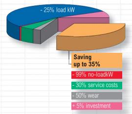
25-35% of the load energy is consumed during idle run without producing air.
